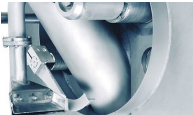
Standard paddle feed control, FC
