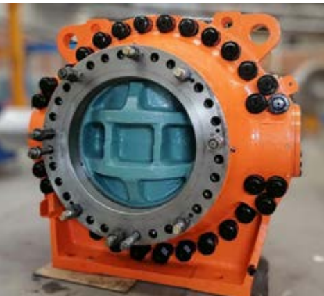
Guatapé hydropower plant, spherical valve DN 1.100 originally manufactured in 1965 and rehabilitated by ANDRITZ Colombia
