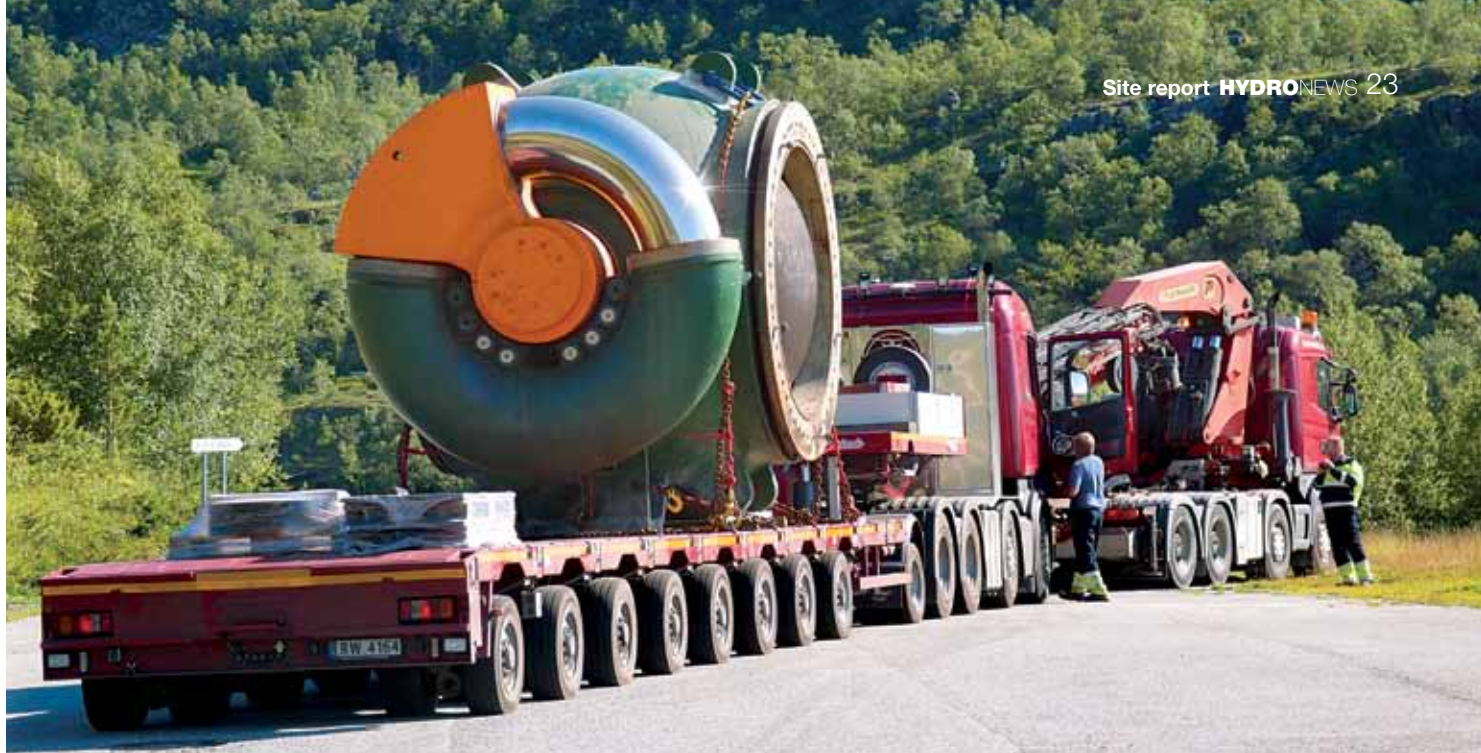
s Transportation of one of the four valves
