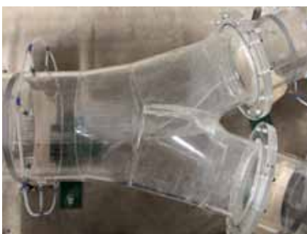
t Bifurcator model test at HPP Pirris, Costa Rica
