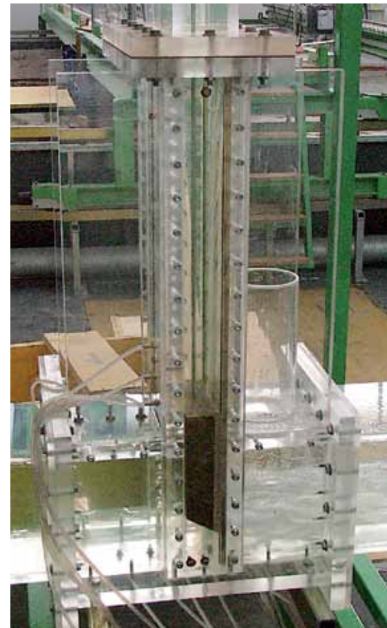
t Intake gate model test at HPP Tsankov Kamak, Bulgaria
