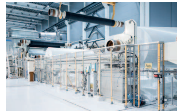
PrimeWinder Arcus Evo and PrimeReel section: The reel's primary arm is equipped with spool weight compensation, and the whole turn-up process is fully automated.
