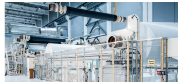
Fully automated tambour change that minimizes maintenance.
