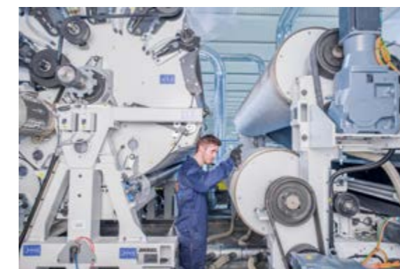
梳理机易打开进行维护
