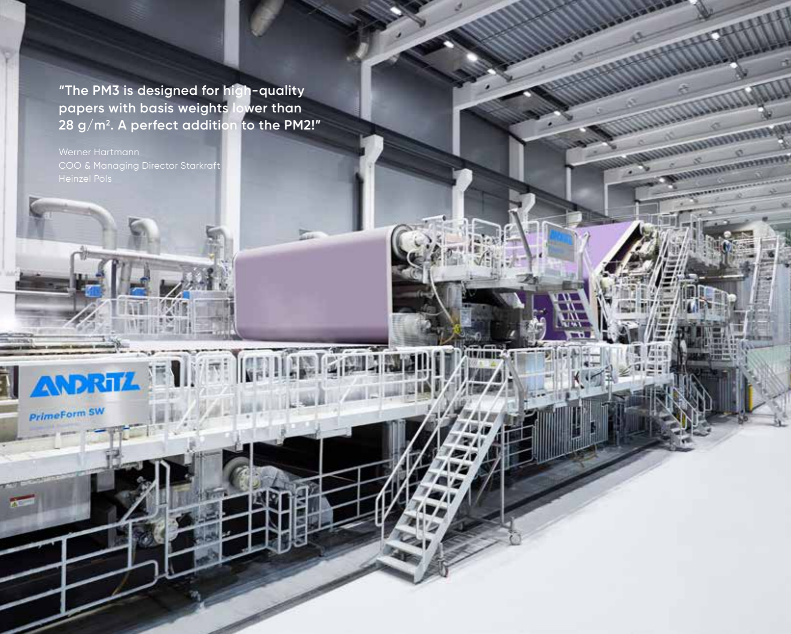
The new PM3: an ANDRITZ solution from the headbox to the reel, including stock preparation, automation and pumps
