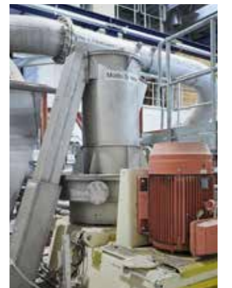
ModuScreens TD tailing screens are part of coarse screening. Efficient washing of fibers is done with a FibreWash Drum – one important part of the detaching system.
