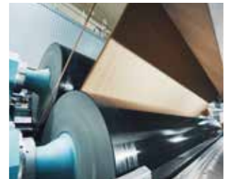
The PrimeFilm film press applies starch simultaneously to both sides of the paper web in order to achieve the desired strength values at high speed.
