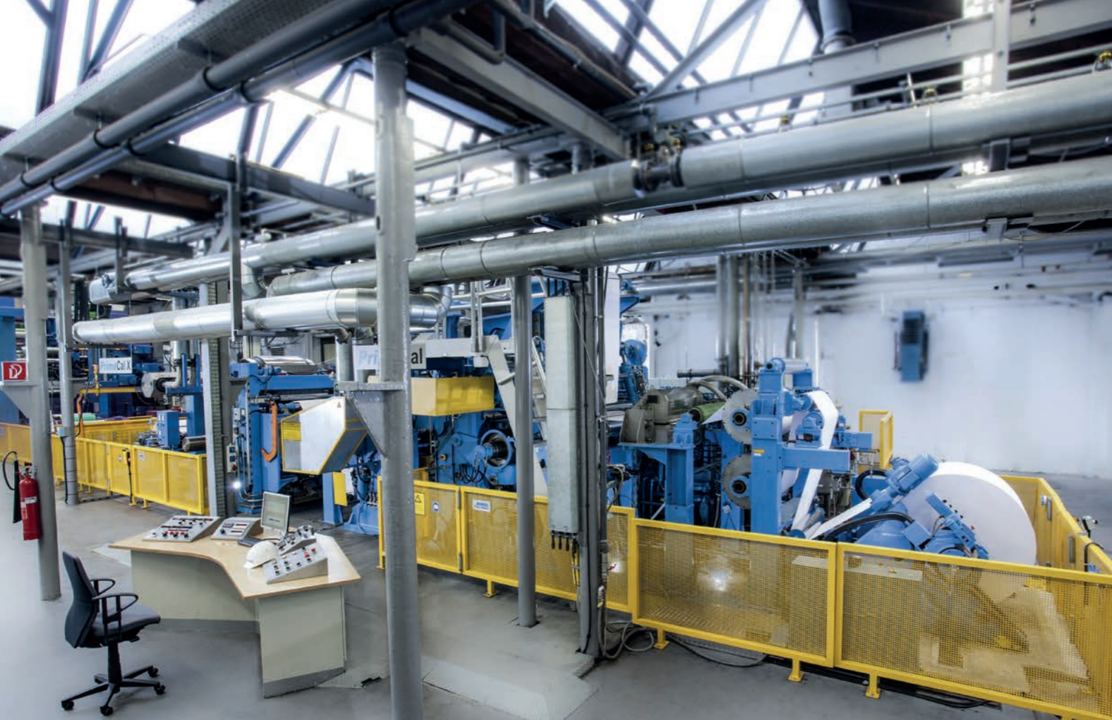
At the Paper Technology Center in Krefeld, Germany, you can choose between our PrimeCal Hard/Soft calender, PrimeCal X shoe calender, and PrimeCal Y belt calender, which can be configured in many ways to take papermaking to a new level. The pilot plant is available for running trials of printing/writing papers, special papers, cartonboard, and packaging grades with its 2x2 or 8+5 rolls and a maximum speed of 1,500 m/min at a surface temperature up to 220° C.
