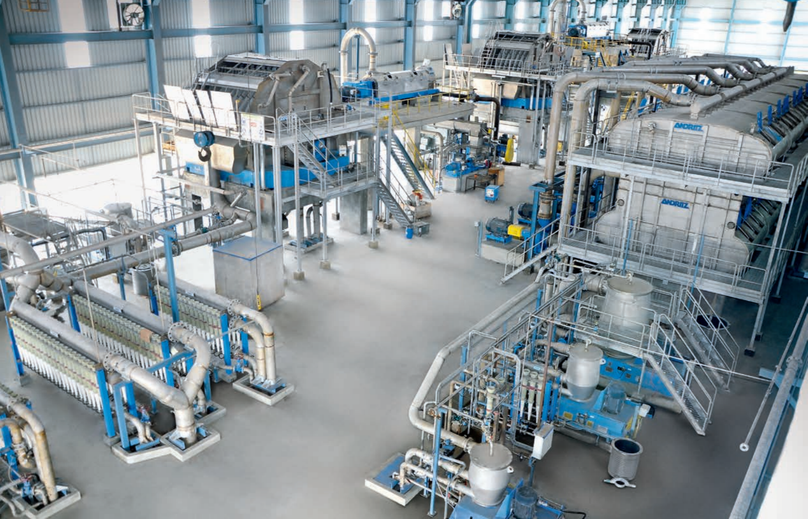
Full range of recycled fiber technologies for the production of excellent stock for various paper grades; modern deinking lines; state-of-the-art systems processing low-quality waste paper to produce high-quality packaging grades.
