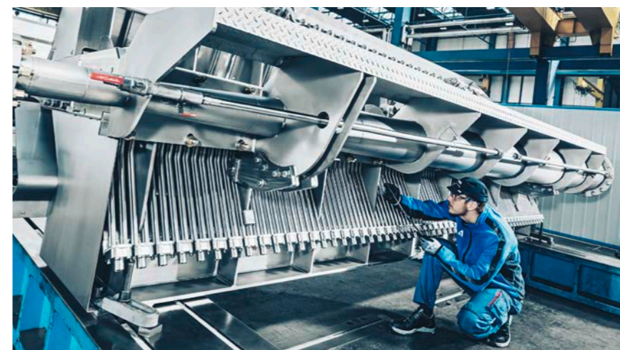
PrimeFlow AT headbox at the ANDRITZ workshop in Austria. The headbox provides excellent jet quality, fiber dispersion and fiber orientation control over a wide range of grades and speeds.
