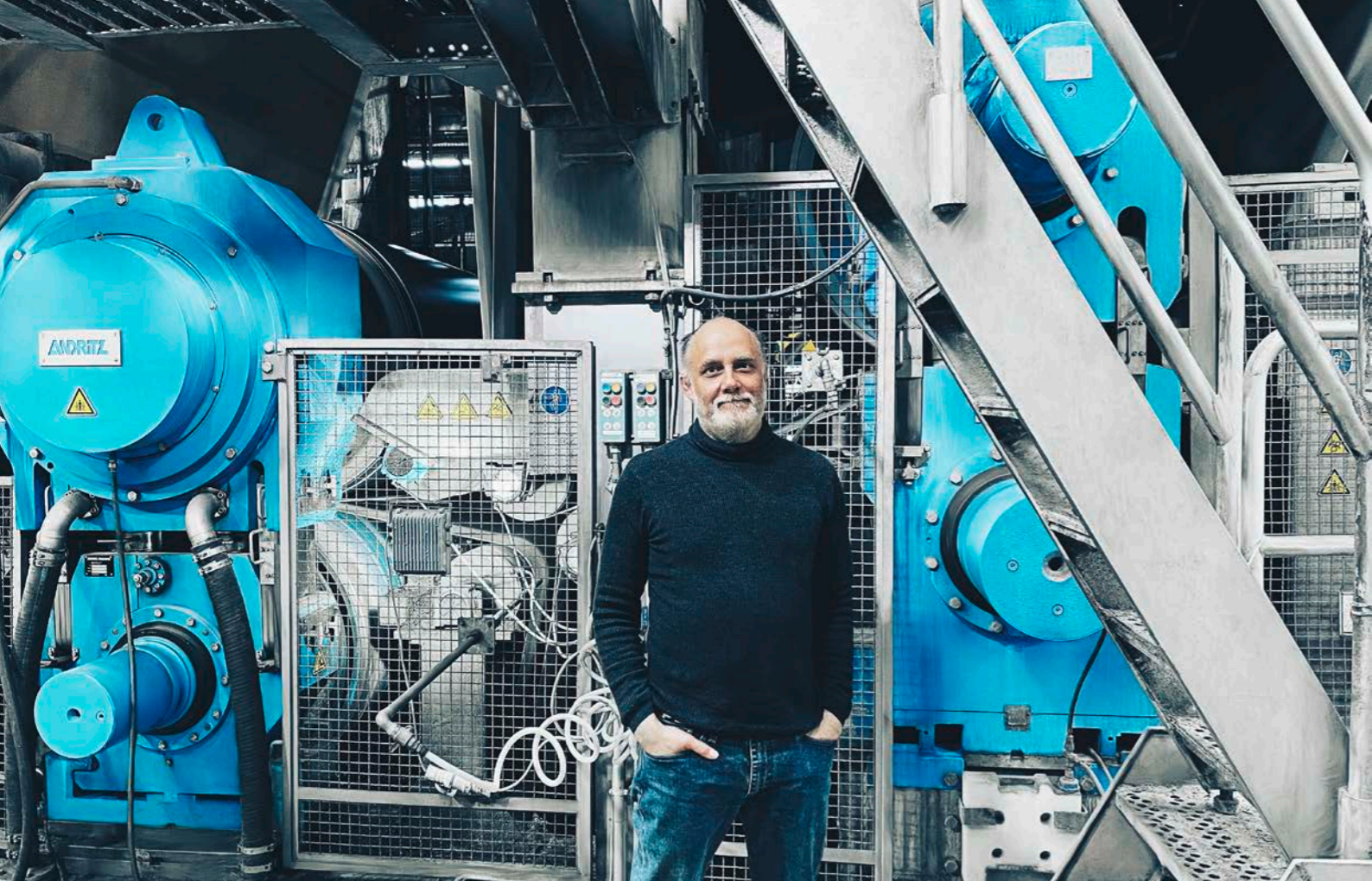
The new PrimePress X shoe press at Merati's BM1 (Italy) is operating at a line load of 2,000 kN/m – a world record! It enables Merati to achieve extraordinary dry contents of up to 59%. In addition, the runability of the machine increased and the specific energy consumption decreased significantly. Photo: Marco Merati, Managing Director, A. Merati & C. Cartiera di Laveno
