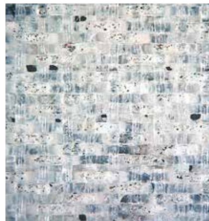
Bag plugged due to insufficient cleaning
