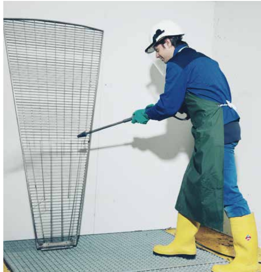
High-pressure cleaning of sector
