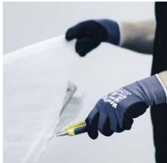
Disassembly of disc filter sector, removal of old filter bag
