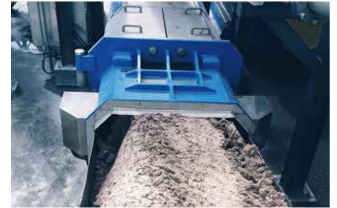
Fine rejects output from the ANDRITZ Reject Compactor
