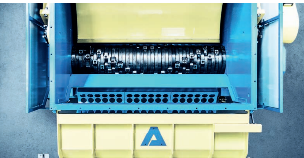
Top view of an ADuro U shredder – for innovative one-step shredding to a defined particle size
